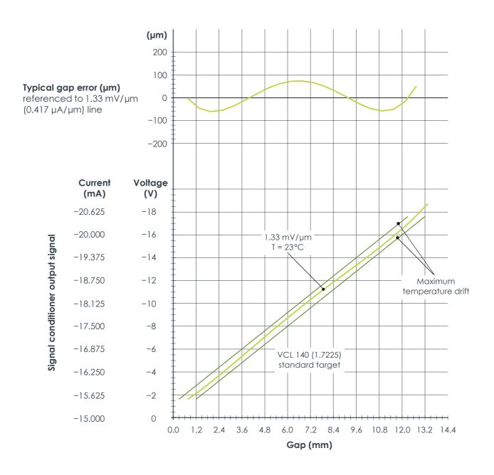
Proximity transducer:TQ403Signal conditioner:IQS900Standard target material:VCL 140 (1.7225)Equivalent materials:A 37.11 (1.0065), AFNOR 40 CD4, AISI 4140
